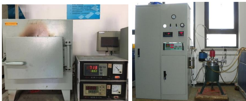
Fig 1. The picture of muffle furnace (left) and pressure-resistant autoclave (right) used in experiment
