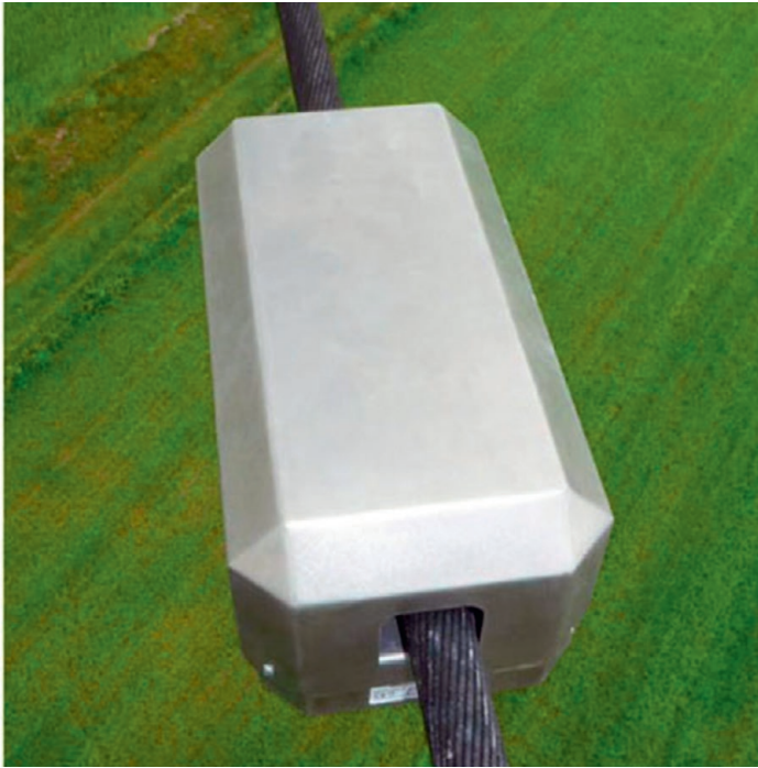
Photo 1. Photo of a logger on a 400 kV line wire [9]
