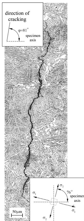
**Fig. 12. Fatigue cracking in the specimen tested at  $S_{eq} = 532$  MPa recorded after  $N_i = 4.1 \cdot 10^4$  cycles.**
