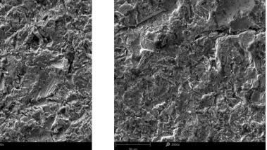
Fig. 8. Photographs of the surface of samples (magnification 2000×): 38GSA – a) 30°, b) 90°; Hardox 500 – c) 30°, d) 90°
