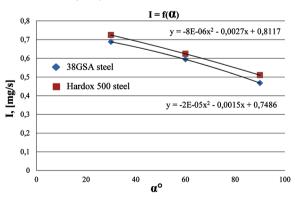
Fig. 7. Correlation between the erosion rate *I* and the impact angle of particles
