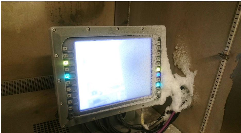
Fig. 1. Monitor unit during climatic tests
