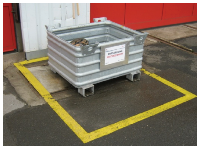
Fig. 9. Example of floor marking for storage boxes [photo by the author]
