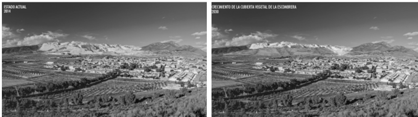
Fig. 23 Simulation of the possible landscape evolution at Pinoso marble quarries (Alicante). To do this, two-dimensional computer graphics from an image taken from one of the observation points defined as major in the visual analysis have been used Source: CERCLE & Alba Consultores, S.L. Technical documentation .
