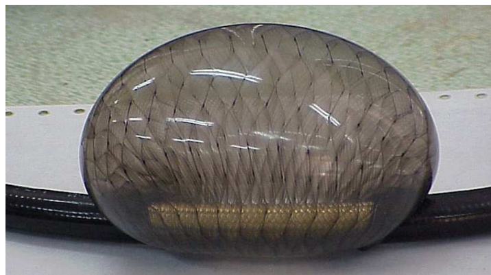
Fig. 14 A case of delamination of a braid made of plastic from a metal braid of a pressurised, flexible diving system hose.
