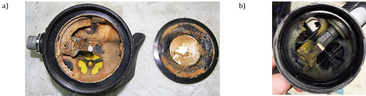
Fig. 5 Examples of contamination of a 2nd stage of a breathing apparatus [8,12].
