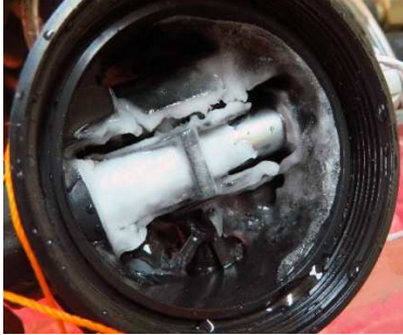
Fig. 13 Examples of freezing of elements of diving equipment: a) 2nd stage of a breathing apparatus used in water with a temperature of approx. 4 °C; b) filter integrated in the shut-off valve of the exhaust system of a decompression chamber.
