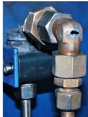
Fig. 10 Damage to diving equipment components resulting from a sudden event:
