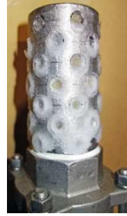
Fig. 13 Examples of freezing of elements of diving equipment: a) 2nd stage of a breathing apparatus used in water with a temperature of approx. 4 °C; b) filter integrated in the shut-off valve of the exhaust system of a decompression chamber.
