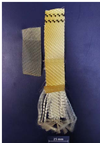
Figure 11. Example of a hose tape sample subjected to a delamination force test, the PVC inner lining of which has ruptured
