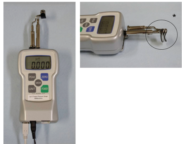
Fig. 1. A perioral muscle pressure measuring device with a lip piece (Lip & Tongue Pressure Gauge ® ).
