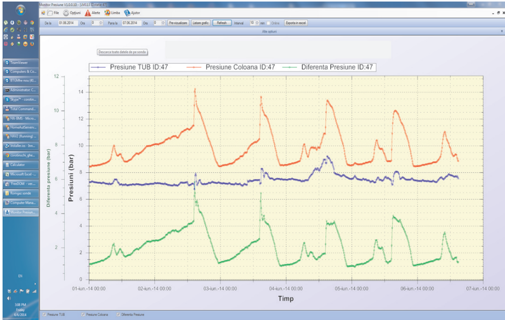
Fig. 5. Tubing and casing pressure report chart for one well
