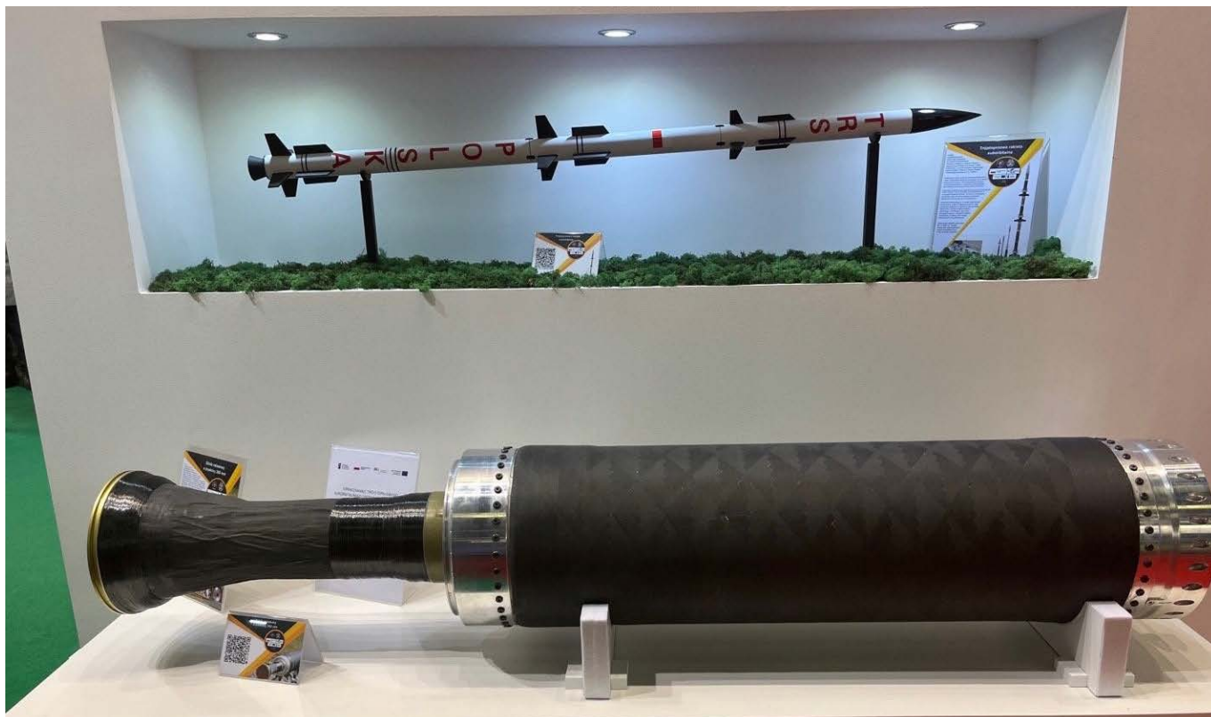
Figure 6. Three-stage rocket solid rocket motor with its blast tube type nozzle shown at MSPO 2022 event
