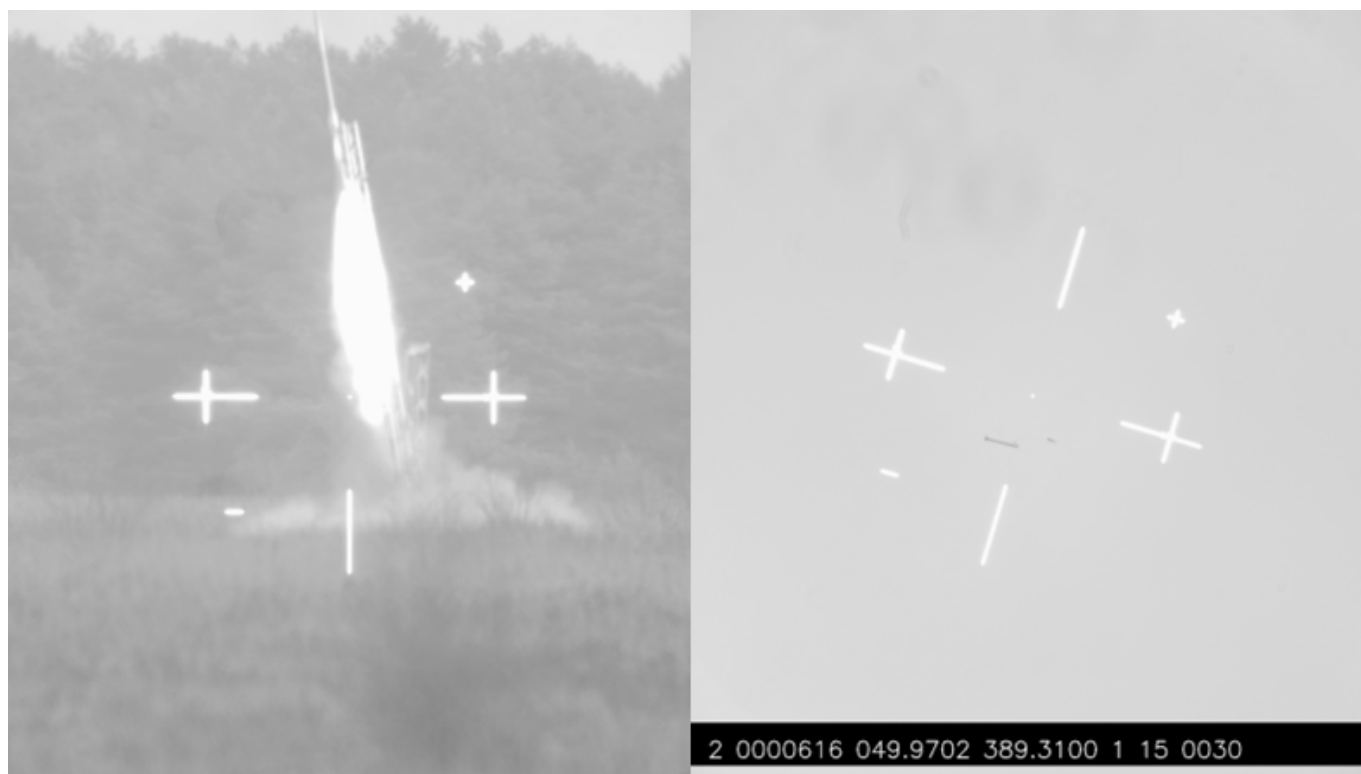
Figure 3. Cinetheodolite frames from the recording of the flight. On the left: lift-off event; on the right: separation of the recovery system
