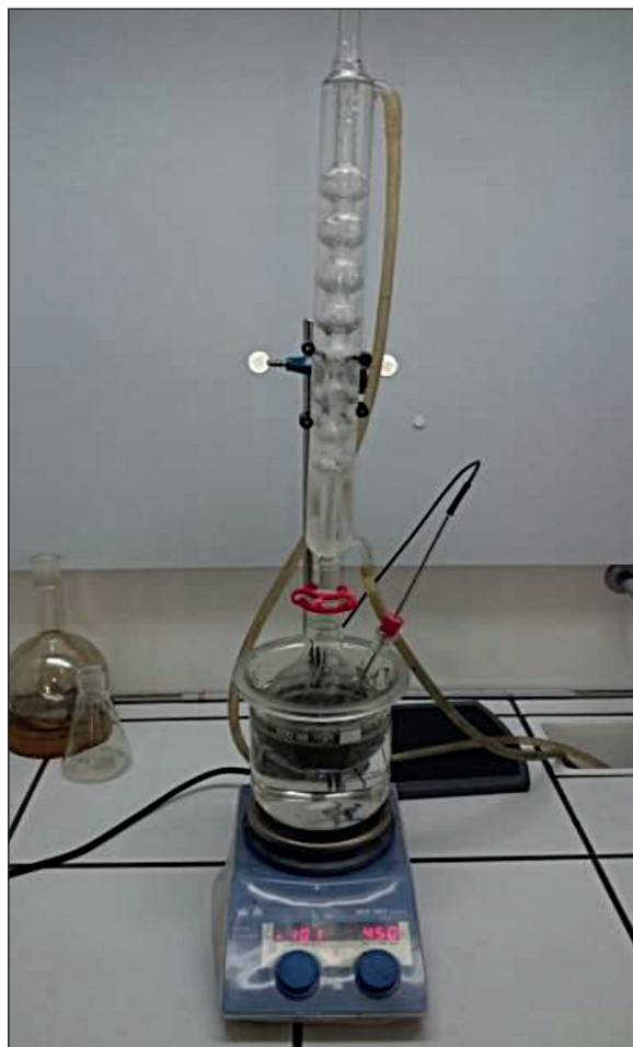
Figure 1. Laboratory set-up for the zeolitization of combustion by-products
