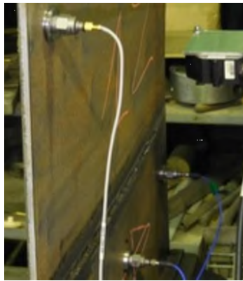
Fig. 3. A photo of one of the tested boards with measuring sensors installed
