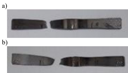
Fig. 1. Weldments after tensile testing: a) specimen S1; b) specimen S4
