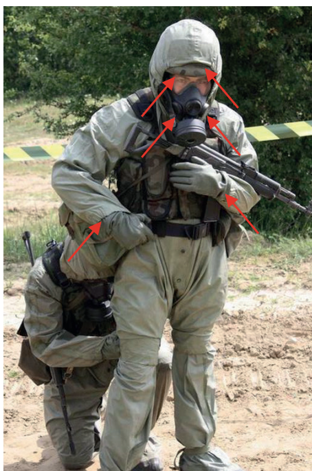
Fig. 3. Possible areas of CWA vapor transmission under protective clothing Source: Own study based on [6].
