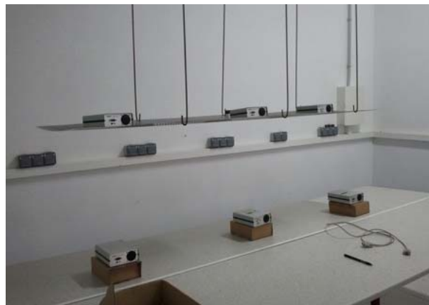
Fig. 3. Position of Radon Scout monitors used during the interlaboratory exercises to obtain reference levels of radon exposure.
