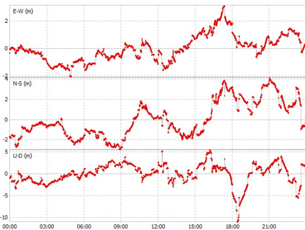
Figure 7. GPS+GLONASS, with broadcast ionospheric correction
