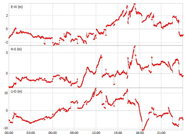
Figure 4. GPS-only, without ionospheric corrections
