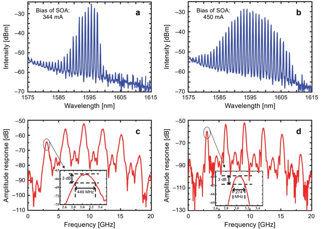
Fig. 2. Measured optical spectra of multiple taps: the bias of SOA is set as 344 mA (a) and 450 mA (b). The corresponding frequency responses of the multi-tap bandpass MPF (c, d). Inset – the zoom-in view of the first passband.
