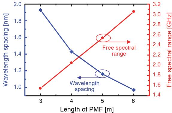
Fig. 5. Wavelength spacing of the multiple taps and FSR of the multi-tap bandpass MPF with different length of PMF.
