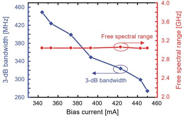
Fig. 3. The 3-dB bandwidth and FSR of the MPF with different bias of SOA.
