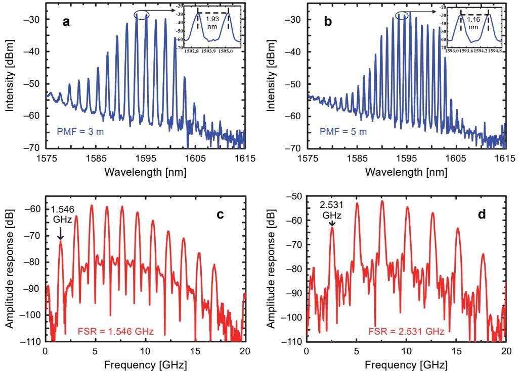
Fig. 4. Measured optical spectrums of multiple taps when the lengths of PMF are 3 m (**a**) and 5 m (**b**). The corresponding frequency responses of the multi-tap bandpass MPF (**c**, **d**). Inset – the zoom-in view of two arbitrary adjacent optical taps.
