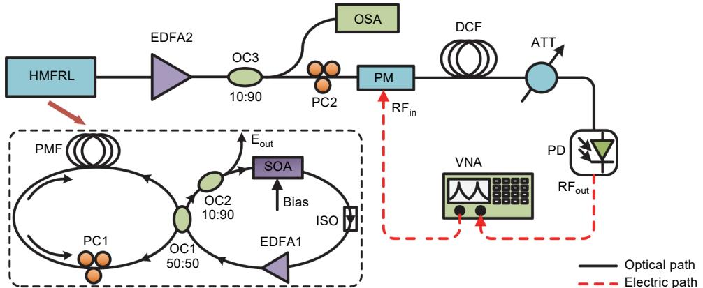
Fig. 1. The schematic diagram of the proposed MPF. PMF – polarization maintaining fiber, PC – polarization controller, OC – optical coupler, SOA – semiconductor optical amplifier, ISO – isolator, EDFA – erbium-doped optical fiber amplifier, OSA – optical spectrum analyzer, PM – phase modulator, DCF – dispersion compensating fiber, ATT – optical attenuator, PD – photodetector, VNA – vector network analyzer.
