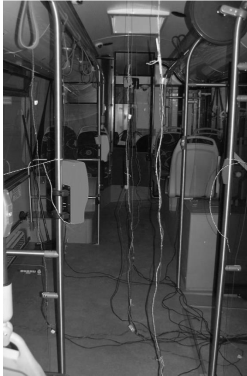
Fig. 3. Sensor grid of installed transducers inside the vehicle
