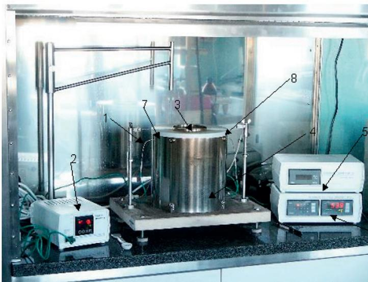
Fig. 7. View of test bench for determining the minimum ignition temperature of the dust layer, where 1 – posts for mounting, tensioning and adjusting the height of position of measuring thermocouple, 2 – heating plate temperature regulator, 3 – ring with sample of tested dust, 4 – furnace body, 5 – control thermocouple, 6 – computer temperature recorder, 7 – measuring thermocouple, 8 – heating plate
