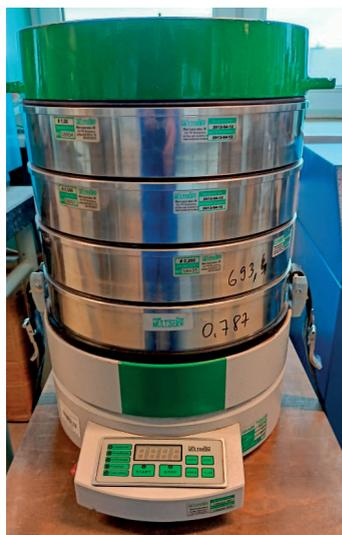
Fig. 3. View of vibrating sieves used for sieve analysis
