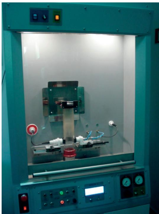
Fig. 6. View of the test rig for determining the minimum ignition energy of air-dust mixtures
