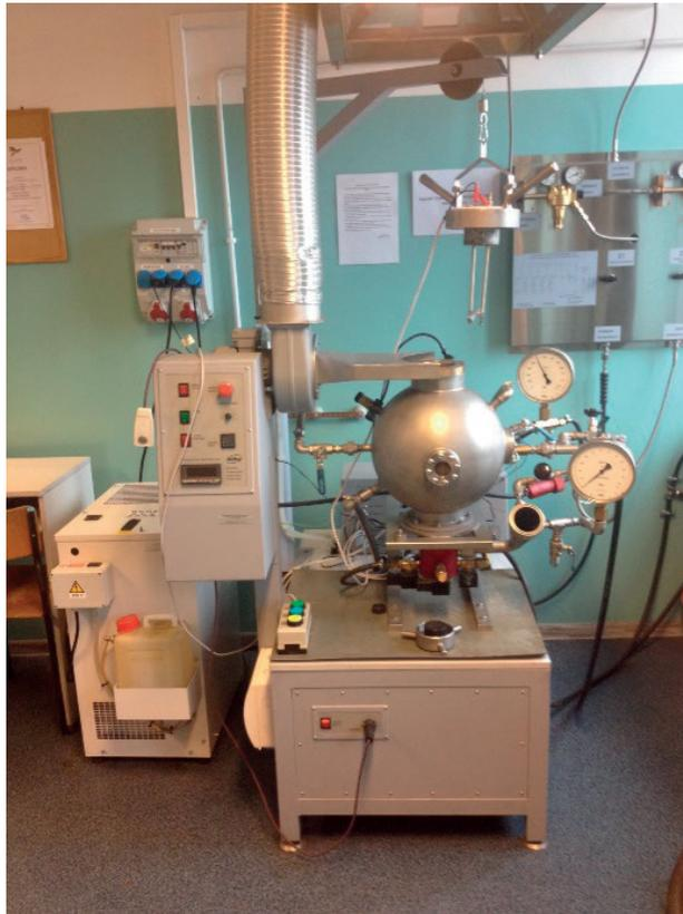
Fig. 5. View of the test stand for determining the explosive characteristics of dust clouds
