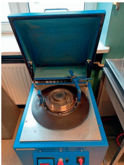
Fig. 2. View of Testchem's LMW vibrating mill
