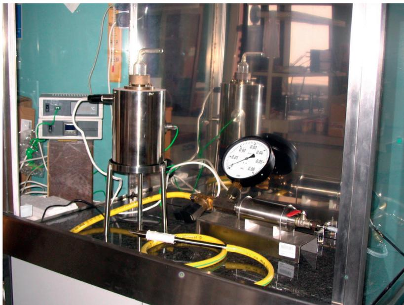
Fig. 8. View of the test rig for determining the minimum ignition temperature of a dust cloud – Godbert-Greenwald furnace
