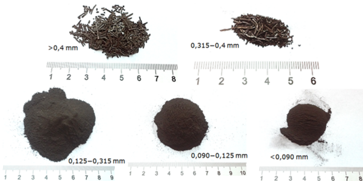
Figure 8. Fractions of pyrolyzed and ground tantalum capacitors
