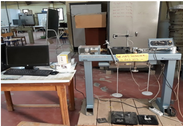
Figure 5: View of the direct shear box apparatus.
