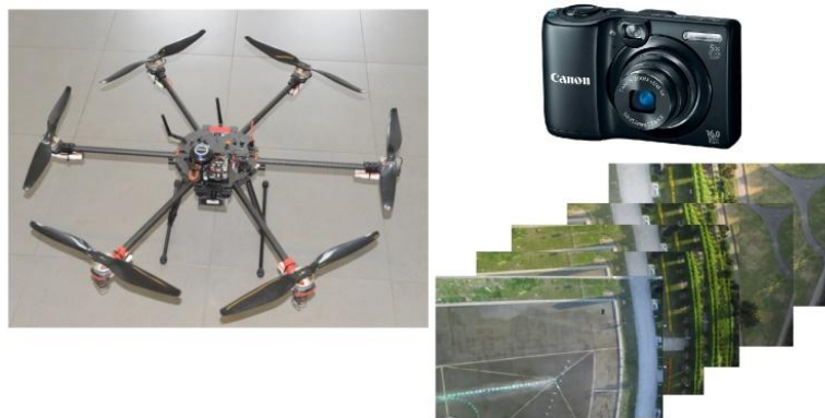
Fig. 2. The low-cost self-made hexacopter RPAS platform and applied compact digital camera that were used in this experiment, with some image samples.
