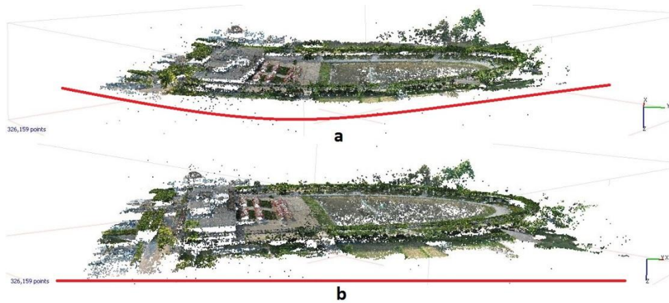
Fig. 4. Dense cloud, (a) without GCPs and (b) with GSPs optimization. The red line shows the systematic error before (a) and after (b) optimization.
