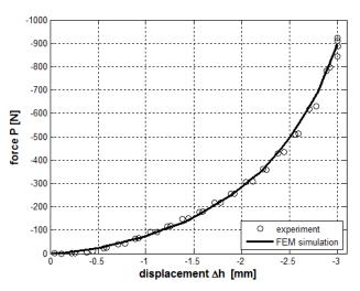
Fig. 10. Comparison of experimental results with the FEM simulation of pressing cylindrical rubber sample into groove
