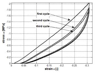
Fig. 5. An example of an elastic histeresis for a tested rubber sample
