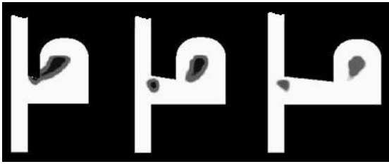
Fig. 6. Influence of the neck length on appearance of shrinkage defects at the neck junction (traditional feeders, cast iron castings)
