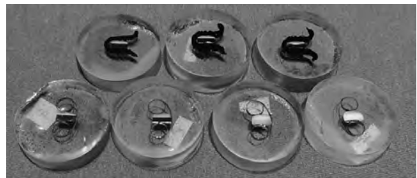
Fig. 2. Specimens for the analysis of layered structures of prosthetic crowns
