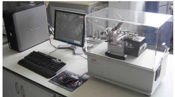
Fig. 2. Wear apparatus (CSM Tribometer)
