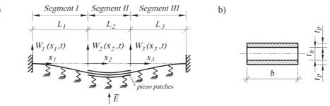
Figure 1. Scheme of clamped-clamped beam resting on elastic Winkler foundation with two piezoelectric patches colocally mounted along the central segment (a), piezosegment cross-section (b)
