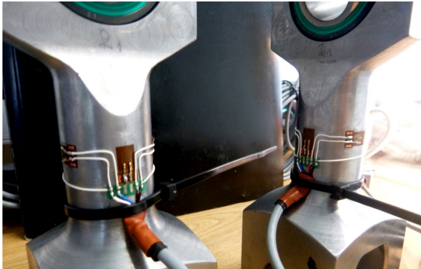
Fig. 3. Strain gage measurement systems without protection against mechanical damage
