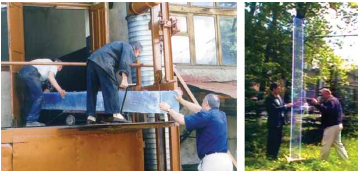
Fig. 1. Sheets of the non-matrix composite of PS base with luminophore o-POPOP ingredient obtained after polymerization at SCI "Monocrystals" Ukrainian National Academy of Science
