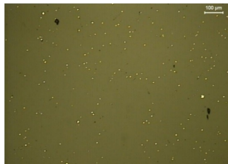
Fig. 4. Agglomeration of the copper droplets in the cooled slag
