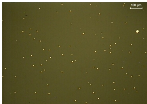
Fig. 7. Agglomeration and coagulation of the droplets in slag
