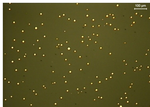
Fig. 5. Agglomeration and coagulation of the droplets in the slag
