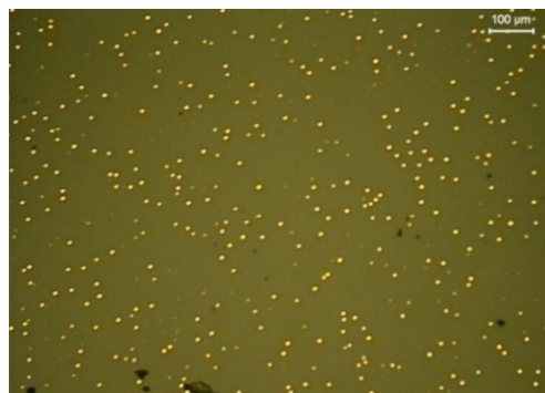
Fig. 6. Agglomeration and coagulation of the droplets in slag
