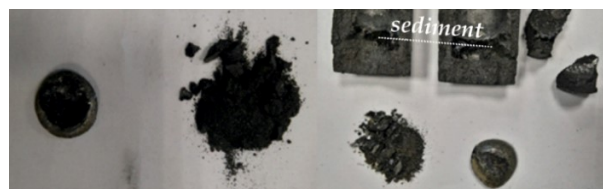
Fig. 9. Copper deposited on the furnace bottom due to activity of both the complex reagent and gravity
