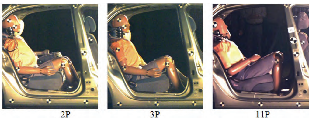
Fig. 2. Initial dummy position in a rear seat of a car ( t = 0 s)
