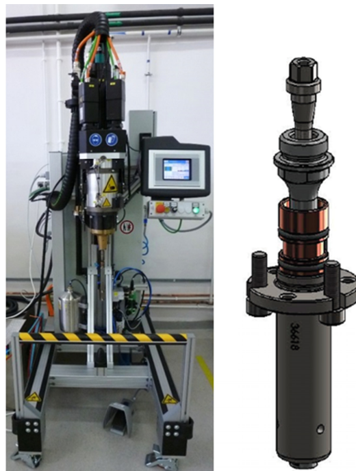
Fig. 1. RPS100 welding machine (left) and RFSSW tool (right)
