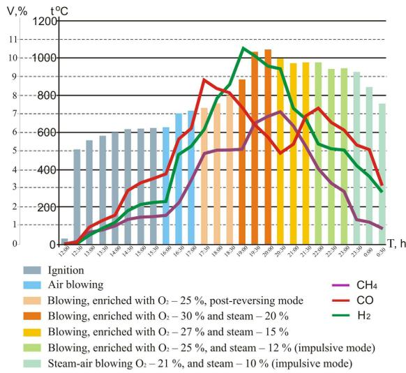
Figure 4. Temperature balance (t) and combustion gases outlet (V) depending of different blowing mixture in a time
