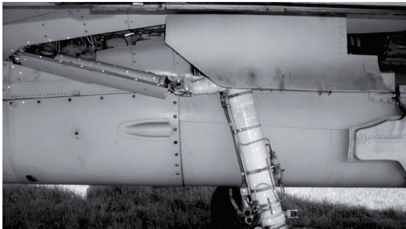
Fig. 2. Markers placed on the examined object (main landing gear of Mig-29 aircraft)
