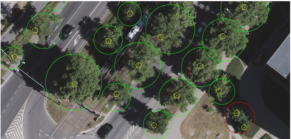
Fig. 5. Automatic tree detection error, in comparison to true situation of trees on base map (yellow)
