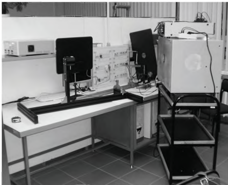
Fig. 3. View of the test stand with a halogen lamp in a special fitting, a xenon lamp in a special luminaire and the integrating sphere
