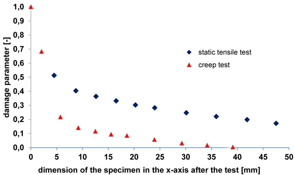
Fig. 2. Damage parameter as the function of the distance from the fracture for a specimen after static tensile test and after creep test.
