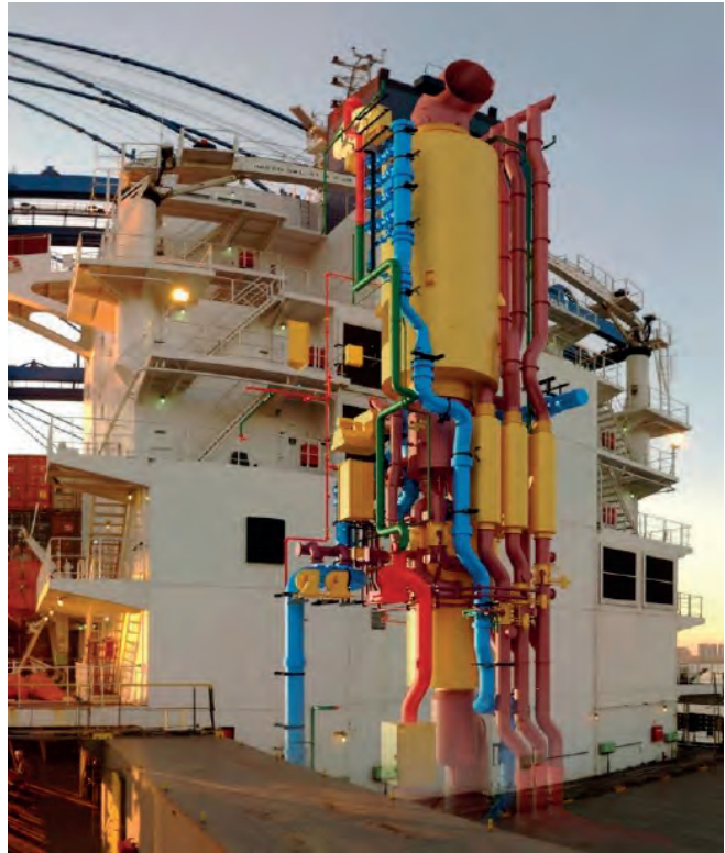
Fig. 1. Visualisation of the BIM model of the exhaust gas system of the cargo vessel
