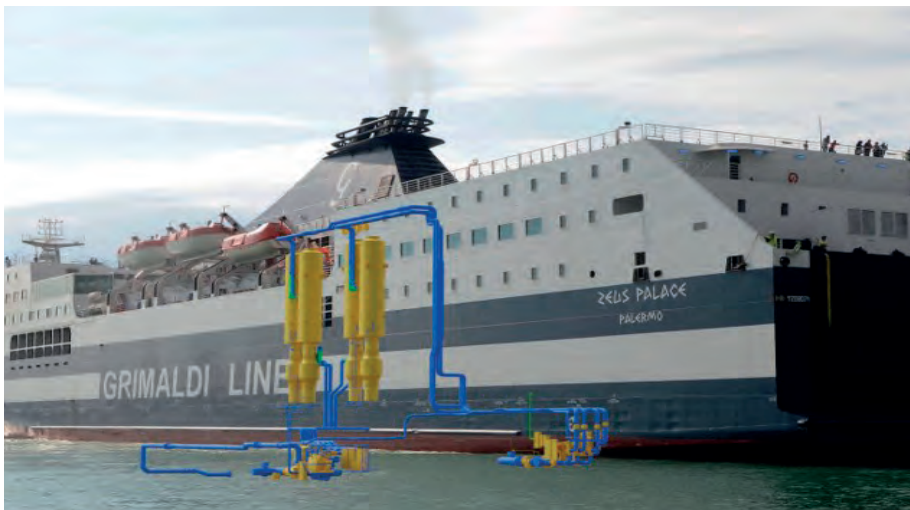
Fig. 2. Visualisation of the scope of a complex multidisciplinary exhaust gas modification for a Ro-Pax vessel
