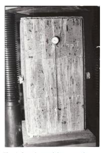
Fig. 1. Sample at axial compression test
