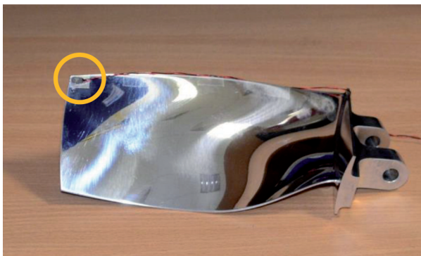
Figure 7. Blade with an attached acceleration sensor at the leading edge (marked with a yellow circle).
