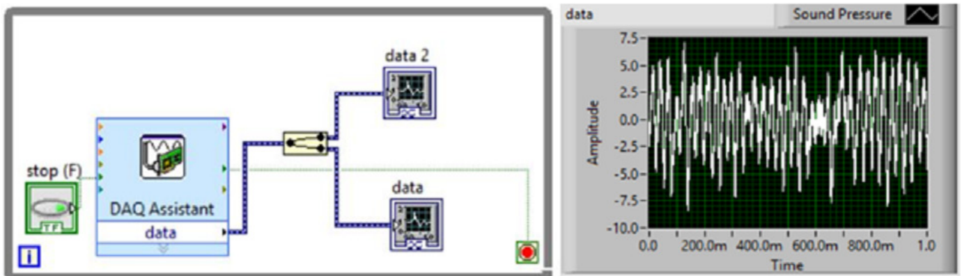
Fig. 4. Lab VIEW program for Data Acquisition
