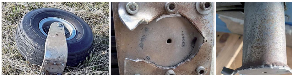
Fig. 8. The separation of wheel from the landing gear [35]
