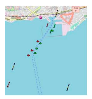
Figure 1. The navigational marking of approach to port of Ystad (South Baltic Four Corners, 2017)
