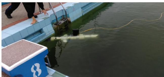
Fig. 3. BUV on tests on pool
