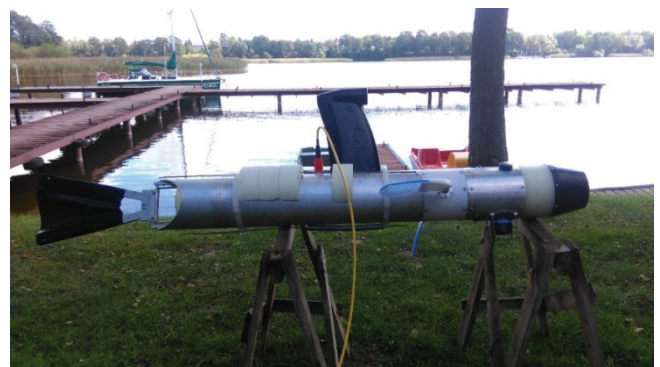
Fig. 2. One of the BUVs built within the project „Autonomous underwater vehicles with silent undulating propulsion for underwater reconnaissance”
