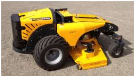
Rys. 11. Zdalnie sterowana kosiarka ROBOZERO. ( www.mcconnel.com/Products/Robocut/ROBOZERO/Default.aspx )
