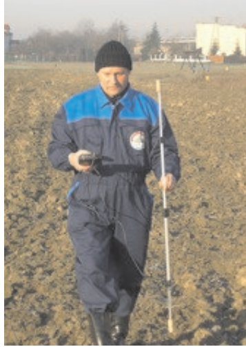
Fig. 2. NCMD measurement on the gas pipeline [2]
