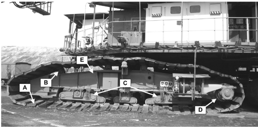
Fig. 1. Basic subassemblies of a large-size tracked undercarriage: A – caterpillar chain, B – supporting wheels, C – balance lever's units, D – driving wheel, E – caterpillar's girder [authors' archive]
