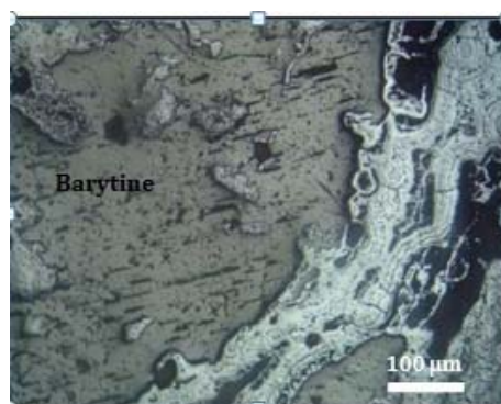
Fig. 6. Barite cracked with triangular pits (NL)
